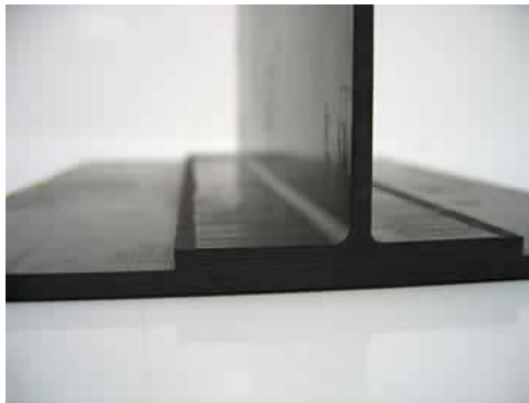
Melding, a Quickstep benefit, melts the surface of one part into the surface of the other making one integrated whole.
